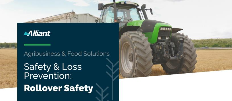
The most frequent causes of tractor-related deaths are side and rear overturns. Because of their high center of gravity, tractors are more susceptible to rolling or turning over than vehicles with a low center of gravity, like passenger cars and trucks. In 1986, Rollover Protective Structures (ROPS) became standard equipment on US-manufactured tractors. However, many tractors manufactured before 1986 are still widely used on farms and unlikely to have been retrofitted with ROPS.
